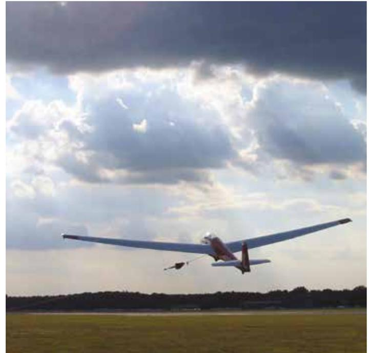
A glider with a 1g stalling speed of 34 knots will stall at about 50 knots during rotation on a winch launch if the rotation rate is 20° per second. The stall speed will be about 45 knots if the rotation rate is 15° per second.
